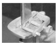
Fig. 11: Use of the screw clamp
