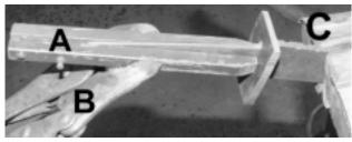
Fig.5: Holding guard in place
